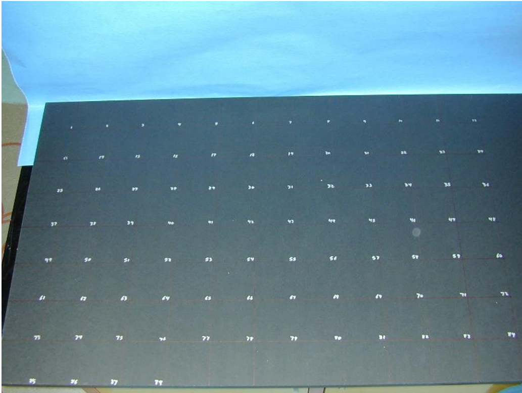
Fig. 1: Overall view of the countertop, divided into 3-inch squares, prior to exposure.
